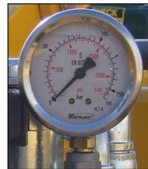
Accumulator Pressure Gauge
